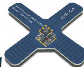
WISP: A Passively Powered RFID Tag with Sensing and Computation
